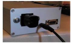
2. Locate the receptacle on the Remote Map Switcher box. Push the other end of the provided cable firmly into the receptacle until it stops.
